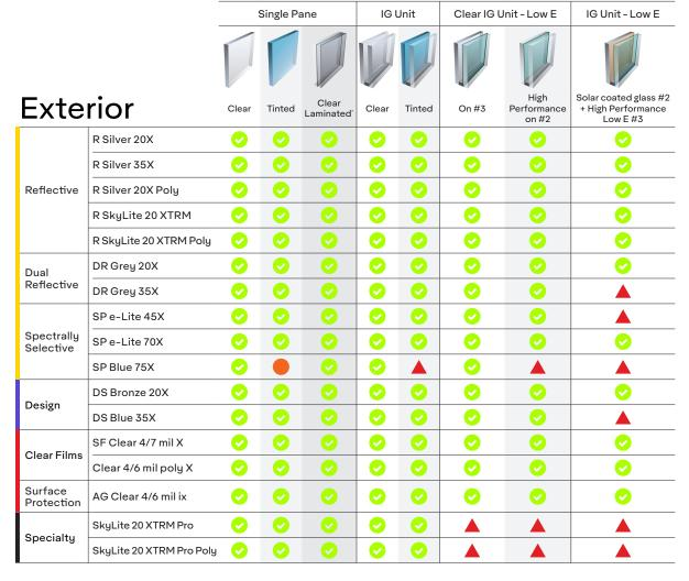
All exterior films require edge sealing. (Some exclusions apply, reference installation guidelines.) For edge sealing it is recommended to use a neutral edge sealing agent such as Dow Corning 791 or 795, Max 5000 by GE or an approved equivalent neutral silicone edge sealing agent specific to exterior applications.
