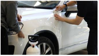
Using the PPF Squeegee Pro Rigid (Blue) or PPF Squeegee Pro Flex (Red), start in the middle of the panel and gradually increase the pressure in order to remove all the air and slip solution from under the film. Overlap the squeegee strokes by about 50% to avoid remaining air/water entrapment.
