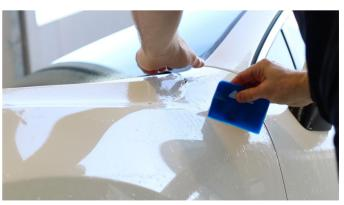
Work from the middle towards the outside edges of the panel, ensuring no slip solution or small air bubbles remain under the film.
