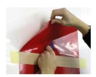
4. Apply the upper portion of the graphic first. Hold the top edge of the graphic smooth and taut away from the application surface with one hand and squeegee horizontally from the centre towards the outer edges. The first squeegee stroke should be just above the hinge where the adhesive has been exposed. Continue squeegeeing, using firm overlapping strokes from the centre out, working away from the starting point.
