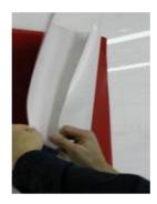
6. Reach behind the graphic and carefully pull the liner back several inches to expose the adhesive.
