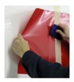
4. Hold the edge of the graphic smooth and taut away from the application surface with one hand and squeegee vertically from the centre towards the outer edges. The first squeegee stroke should be next to the hinge where the adhesive has been exposed. Continue squeegeeing, using firm overlapping strokes from the centre out, working away from the starting point.
