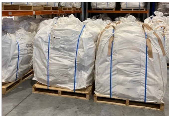
Figure 1: Bulka bag strapped to pallet
