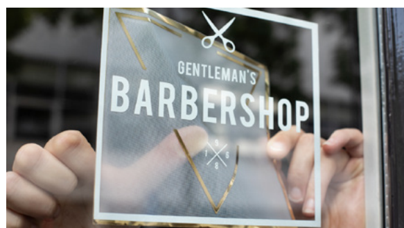
Using Application Tape 300 - High Tack to apply 700PF White and Gloss Gold.
