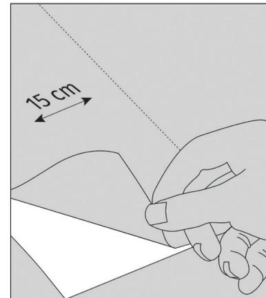
Pull out the backing paper behind Squid® on  $\pm 15$  cm and fold it.
