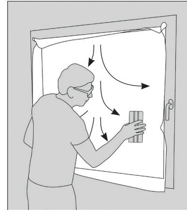
When Squid® is perfectly flat on the window, use the squeegee to adhere it well to the glass. Press from the center outwards (see arrows). Press over the entire surface well, including the edges and the corners.
