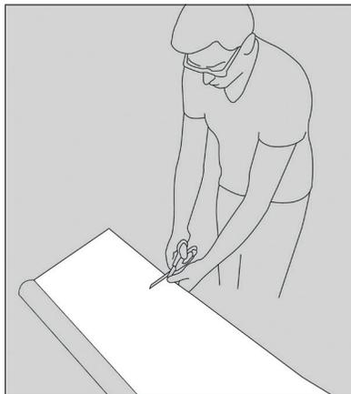
Cut the Squid® somewhat larger than the window, adding  $\pm 5$  cm extra on each side for trimming.
