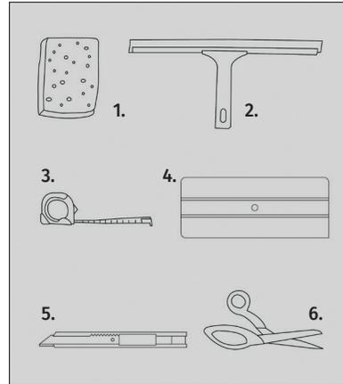
Tools: window cleaning tools (1-2), measuring tape (3), plastic squeegee (4), cutter with stainless steel spare blades (5), scissors (6).
