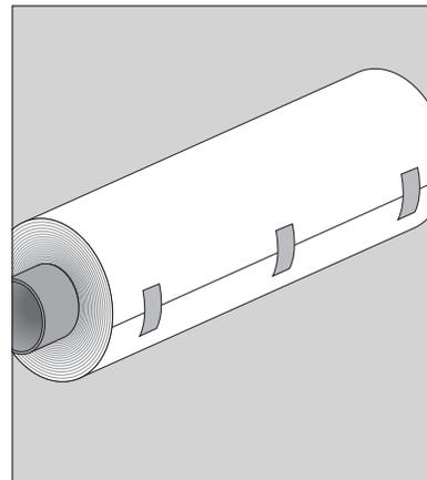
After cutting a piece of Squid®, always make sure to wrap the remaining Squid® tightly around its carton core and fix it firmly with 3 adhesive tapes evenly spread over the width of the roll. If Squid® is not kept tightly enough around the core, this might create permanent bubbles or creases in the fabric.
