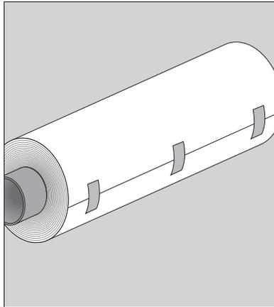
Keep Squid® tightly wrapped around its carton core until the moment of installation. It must be firmly attached with 3 adhesive tapes evenly spread over the width of the roll, in the center, left end and right end.
