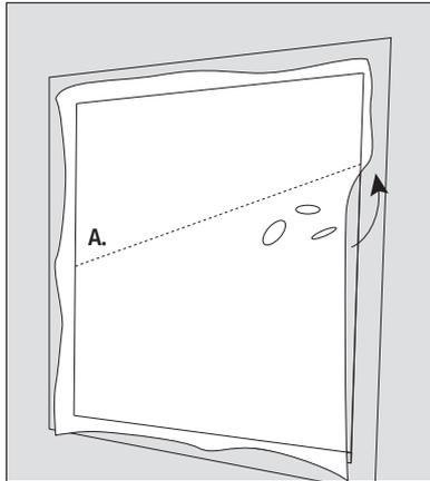
In case of bubble or crease, detach gently the fabric from the window, without applying tension, up to the level beyond the bubble or crease (A).
