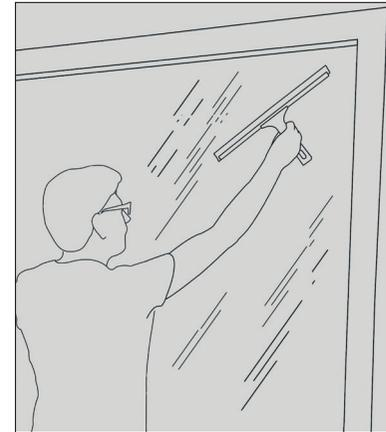
Clean and degrease the window thoroughly with water and a dash of ammoniac or alcohol. Dry the window thoroughly with a lint-free cloth.
