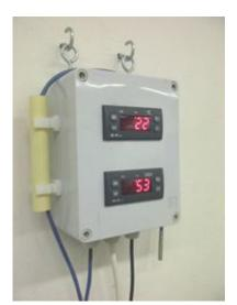
Align climatic conditions in the storage area on one hand and the production area (print or sign cutting) on the other. Difference(s) in humidity and/or temperature level between storage and production can cause the film to react after it has been transferred from one to the other. This can have an immediate effect on media handling.
