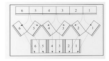
This format of swinging flat surfaces results in matching sides from as many rolls as required of any size sign.
