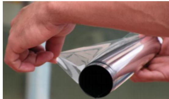
**Step 3 - Precut film:** Precut film to window size, leaving 2cm overlapping edge all around: prepare the film straight from the box, cutting from the hardcoat side with a sharp blade. Make sure the film is rolled with release liner outside (SR coating inside).
