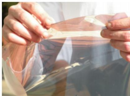
**Step 6 c** - Make sure **NO FOLDING OF FILM TOWARDS RELEASE LINER** occurs, to avoid cracking!
