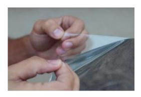
**Step 6a** - Using two pieces of adhesive tape, separate the release liner from the film.
