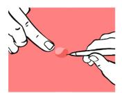
12. The final stage of the application starts. Using the hot air gun, the material should be post heated to a temperature of 175°-194°F (80-90°C), especially in those areas where the material is stretched. The use of an IR Thermometer or IR Heatgun is REQUIRED to ensure you achieve the proper temperature during the post heating process. Make sure that the heating is done gently, and the temperature is gradually increased.
