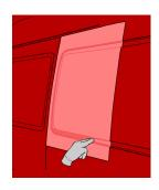
11. Check the application for remaining bubbles. If there still are small air bubbles to be seen, these can easily be removed. Just make a small puncture, heat it a little and push the air out.
