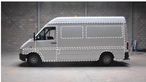
The goal is to clean the entire vehicle and focus especially on the edges, recessed areas, and underneath the body. Edges and recessed areas are the weakest and most vulnerable points for the film and adhesive.
