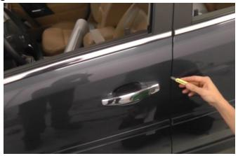
2 - Solid - If the blade is angled away from an edge but doesn't slip behind, it is considered a solid cut. This is because the body of the vehicle continues towards the inside of the vehicle.
