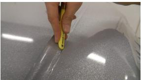
For empty edges that have thicker than normal edges, like on composite body parts or where the film got stretched more than normal, the installer can cut on the empty edge but angle the blade at 180 degrees. To do this, the section being wrapped should be opened. This is called Empty Cut #2. These are commonly found on hoods, doors and trunks.
