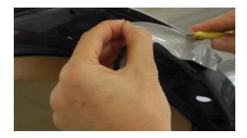
For empty edges that are high grab points or white/yellow/red painted vehicles, its best for the installer to cut on the solid side of the gap. This will create around ¼ inch of material that will wrap around the empty edge. This is called Solid Cut #1. Be sure to heat and soften the angles found on body lines first to avoid any wrinkles when sealing the film onto inside portion of the body.
