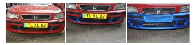
Inlays are separate placements of the film on key areas that work in conjunction with larger sections of film. Inlays help to minimize overstretching and increase the durability of an install. They can be used to help reduce overstretching on deep recessed like on the bumper pictured above or for raised objects that cannot be removed like this door handle.
