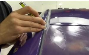
Molding/Roll-up Windows: For windows framed by rubber molding, install the film to the flat surface areas first. This will leave the window perforation bridging the area where the molding is. To safely apply the window perforation, pick it back up and tuck it into the molding that surrounds the window. Be careful when picking the window perforation back up. It is fragile, so pulling too quickly can cause it to tear.
