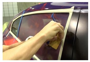
\* Note that the edges of windows surrounded by molding are protected from moisture so there is no need to apply a coat of the edge sealer.
